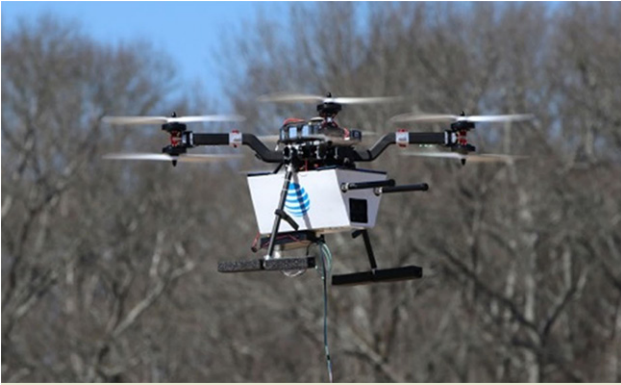
Figure 2 – An example of using a multicopter-type UAV as an aerial platform for relaying communications
