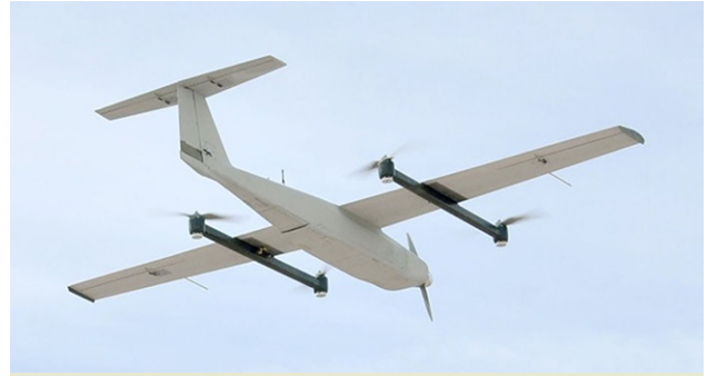
Figure 3 – An example of using a hybrid-type UAV as an aerial platform for relaying communications
