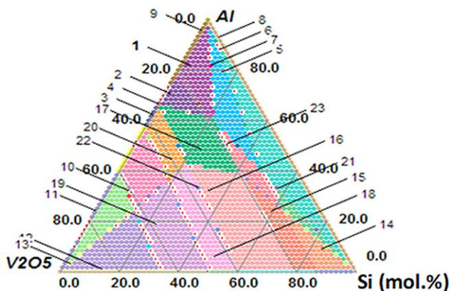
Figure 2 – Three-component phase diagram of  $V_2O_5$ -Al-Si at 400 K
