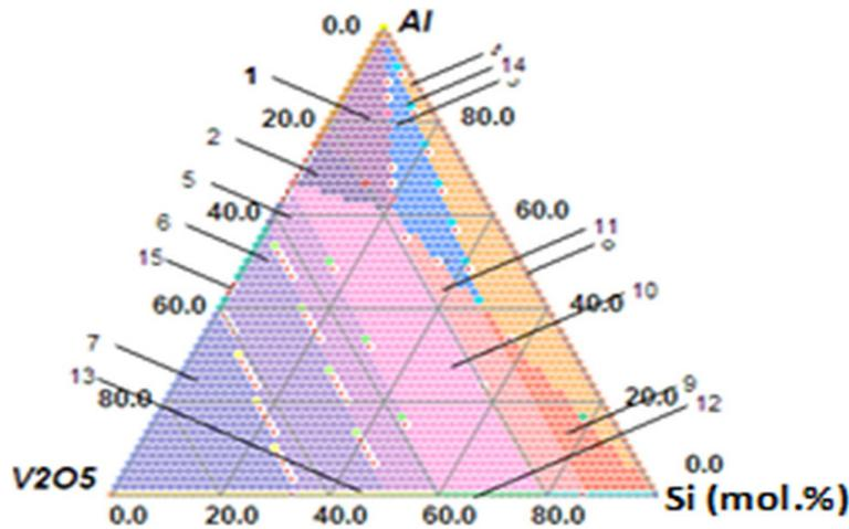
Figure 4 – Three-component phase diagram of V<sub>2</sub>O<sub>5</sub>-Al-Si at 1073 K
