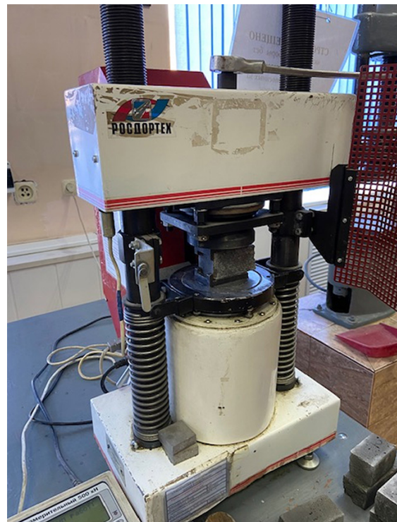
Figure 4 – The process of testing cement beams on a hydraulic measuring press PGN-500
