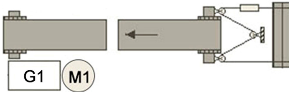
Figure 1 – Kinematic diagram of the main belt conveyor with one drive (M1 – electric drive; G1 – gearbox)
