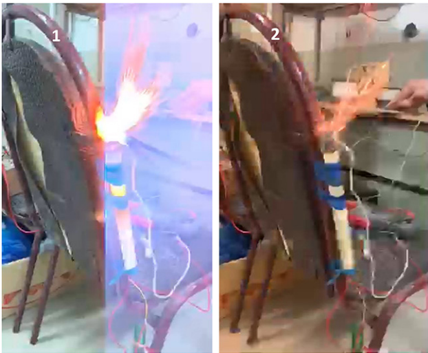
Figure 3 – Completed partial discharge with electrolyte. R_b = 0 , U = 950 V, t = 1/150 s (1); t = 2/150 s (2)
