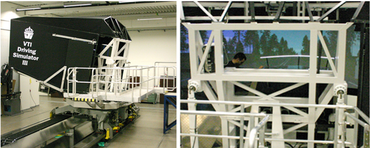
Figure 5 – Hybrid motor platform for VTI simulator (an inside view is on the right)
