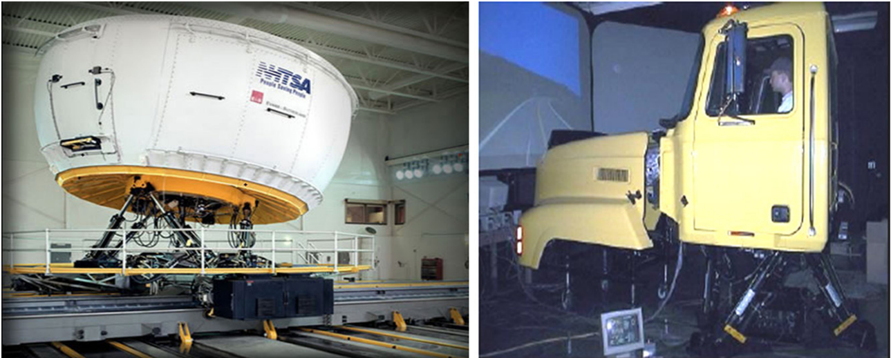
Figure 4 – Advanced system based on the NADS propulsion platform (on the right is a Truck Driving Simulator)
