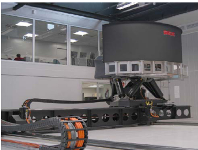
Figure 3 – Advanced simulators on the engine platform in Technocentre Renault (on the right there is the so-called «crossdesk»)
