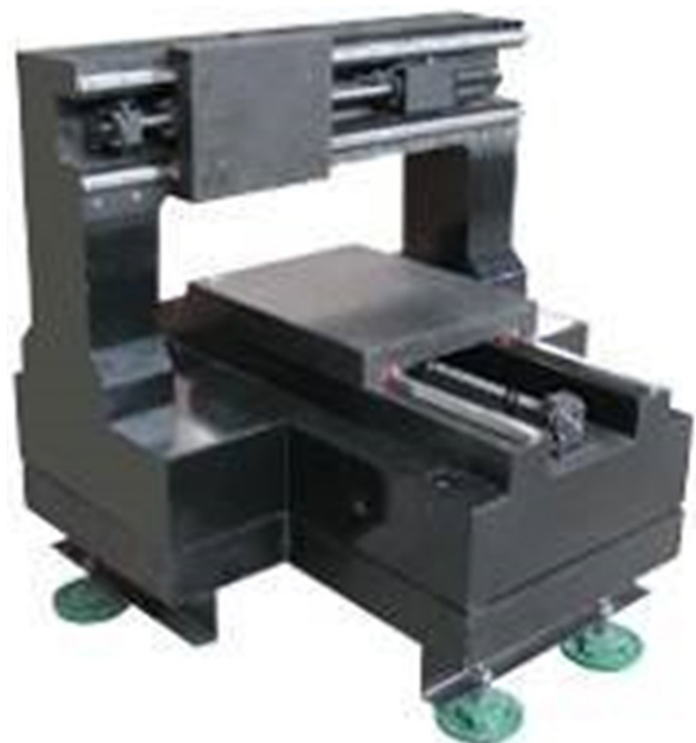
Figure 4 – Metal-cutting machine made of polymer concrete
