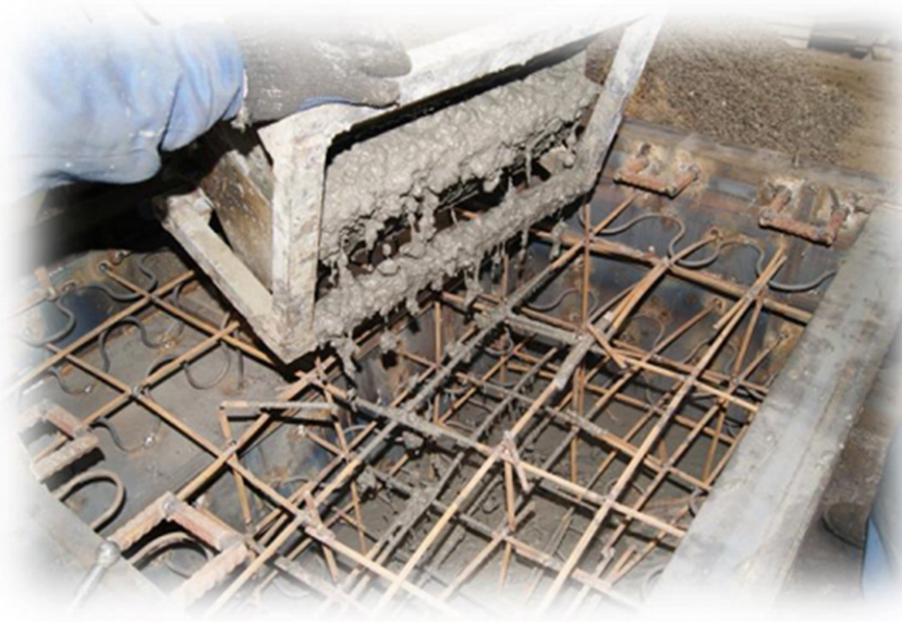
Figure 1 – Manufacturing process of reinforced concrete frame
