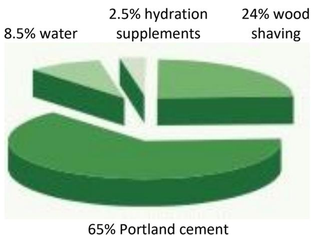
**Figure 1 – Percentage composition of the components in the CBPB production mixture**
