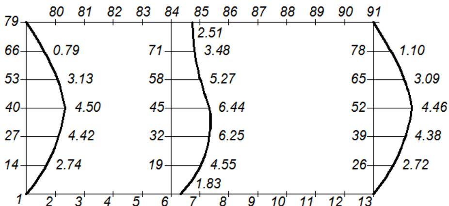
Figure 4 – The value of deflections of the CB when laying out the roof brackets
