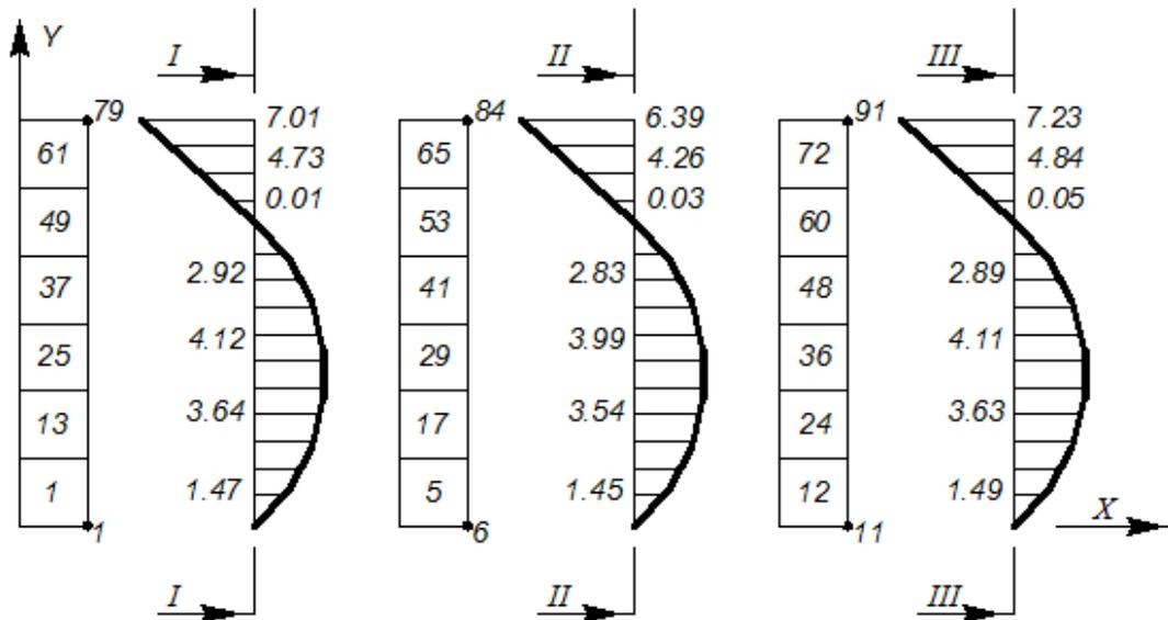
Figure 3 – Plot of the moments when laying out the CB across the roof slope
