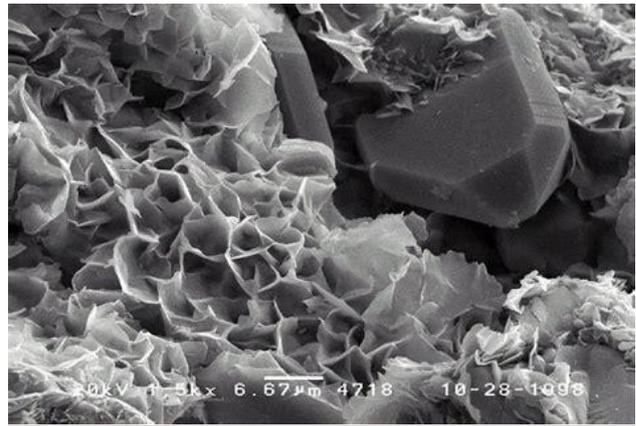
**Figure 1 – SEM (scanning electron microscope) image of montmorillonite – demonstrating the microstructure of smectite minerals that leads to swelling**
