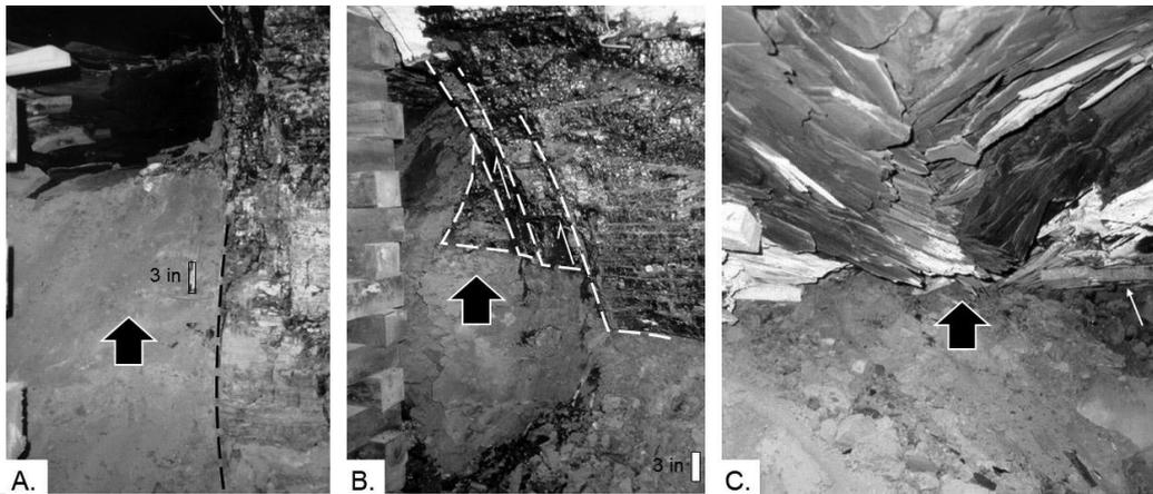
Figure 2 – Photo of soil heaving in a coal mine
