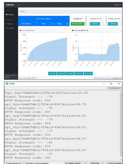
Figure 6 – Curing temperature monitoring
