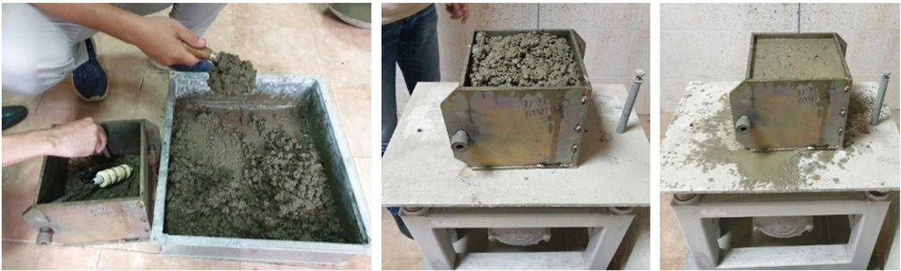
Figure 5 – Concrete pouring into the formwork and vibro-compacting
