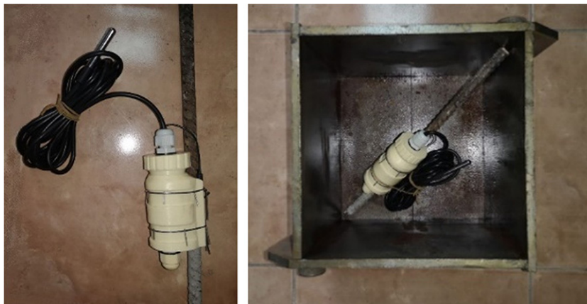
Figure 4 – Installation of the maturity sensor in the formwork
